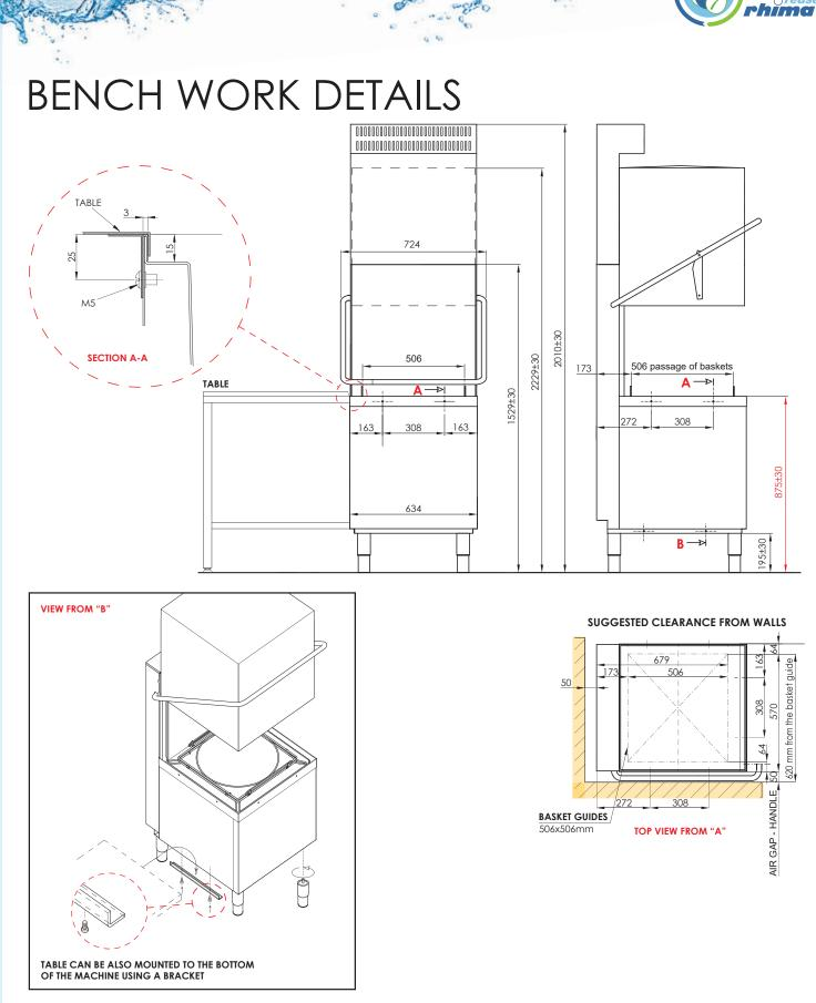
Note: Dimensions shown are a guide only. Benching design/measurements may vary depending on individual site requirements. Rhima suggests final bench design is done with washer in place.
