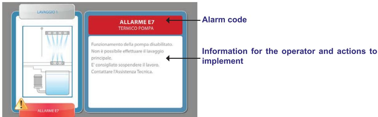
If the alarm does not block the machine it is possible to continue the operation by pressing **RETURN**
