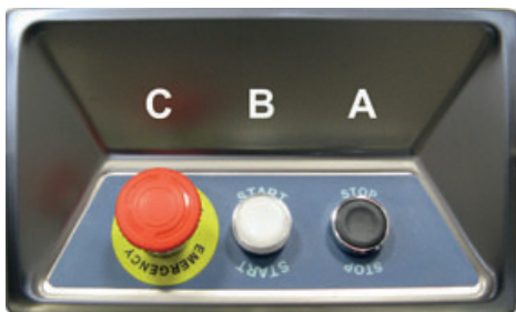
photo 1 A = STOP B = START C = EMERGENCY STOP
