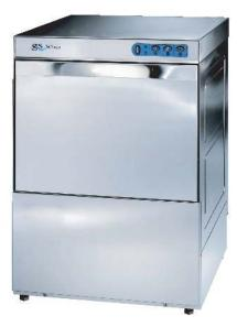
The GS-50ps is a dual cycle feature packed budget priced solution. It is powerful, compact and takes the standard 500 x 500mm rack. The GS-50ps has a drain pump - this means that the machine can be installed in places where the actual waste connection is above the machine outlet point. (Maximum height of 40cm).
