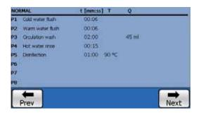
**NOTE!** The cycle variables i.e. temperatures, times and chemical dosage volumes, are pre-set and cannot be adjusted prior to, or during the cycle. Possible changes to the pre-set cycles may only be made by using a special code and into the cycle set-up.
