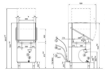
Power supply 400 V Total power 8.7 kW Total current 16 amp Wash tank capacity 15 ltr Rinse water consumption (per cycle) 2.5 ltr Rinsing temp (approx) 80-85 °C Rack size 500 x 500 mm Tallest washable glass 45 cm Weight (empty) 92 kg Water connection 3/4" hose
